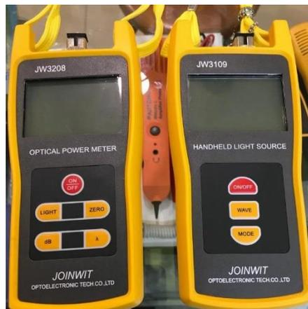
Gambar 2.2 *Optical Power Meter (OPM)*
