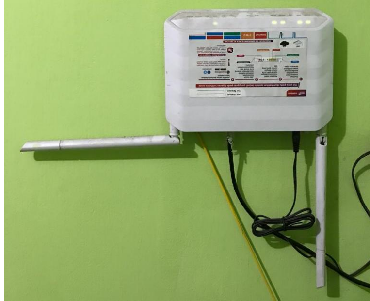
Gambar 2. 10 Optical Network Terminal (ONT)
