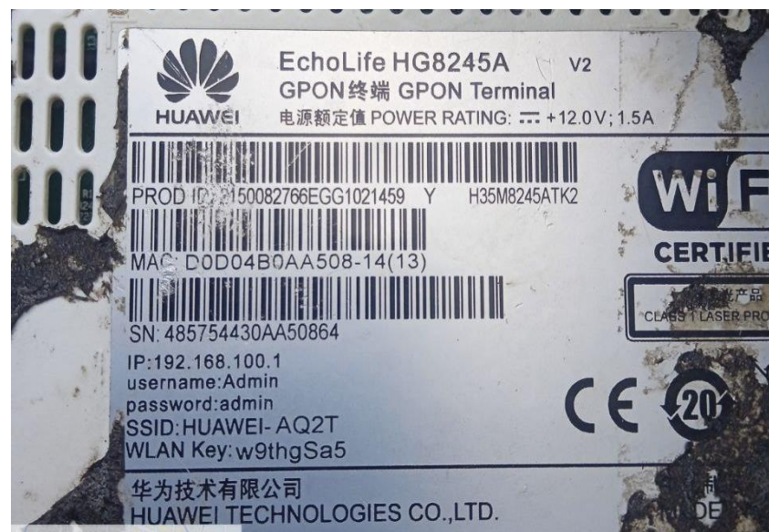
Gambar 2. 7 Serial Number ONT Huawei
