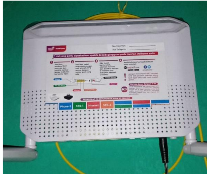
Gambar 2.3 ONT ( Optical Network Terminal ) [3]
