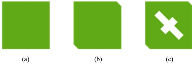
Fig. 1. Stages of the CP patch radiator
