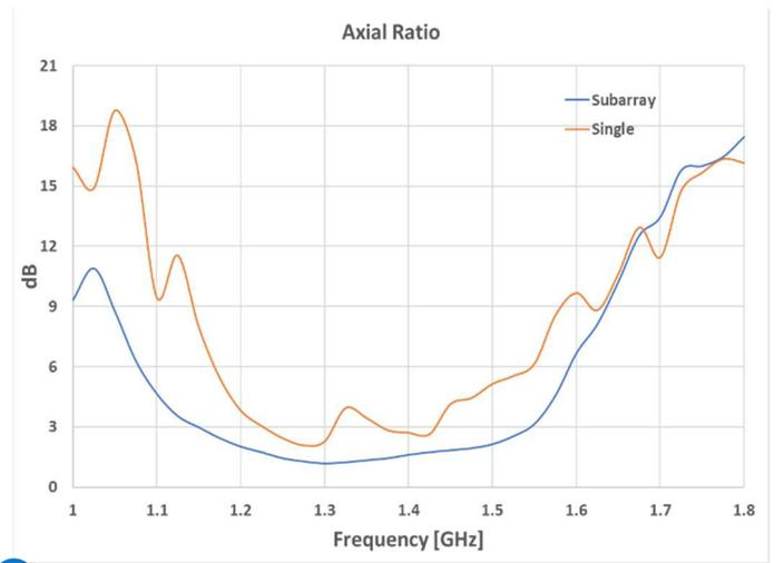
1 Fig. 7. Simulated result of axial ratio
