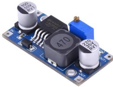
Gambar 2.10 Step Down DC LM2596 [27]
