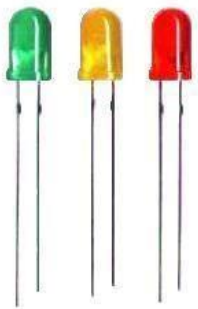
Gambar 2.4 LED ( Light Emitting Diode ) [18].
