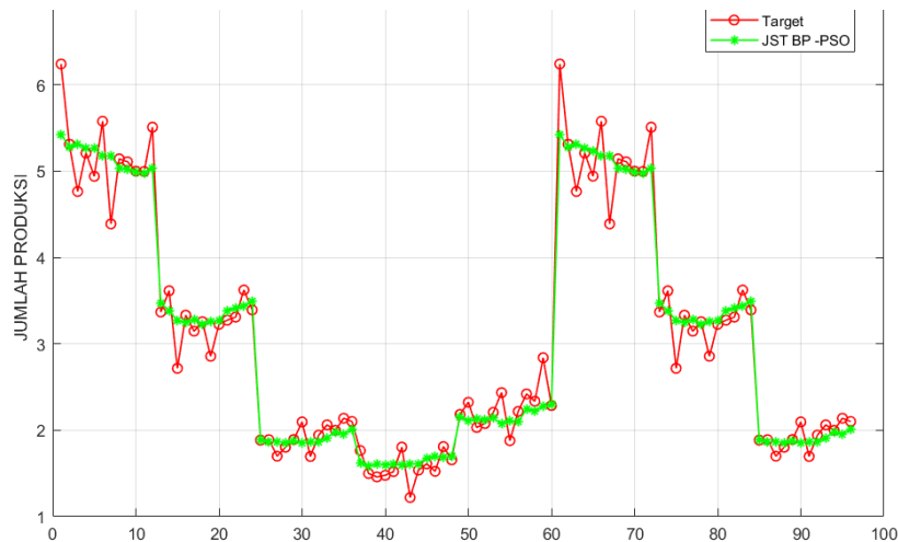
Figure 7. Graph of the train results of the combination of backpropagation ANN and PSO
