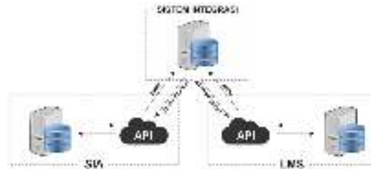
Fig. 1. RESTful Web API Architecture on System Integration
