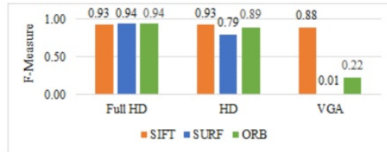
Fig. 9 The experiment result of effect on video resolution toward F_1 value
