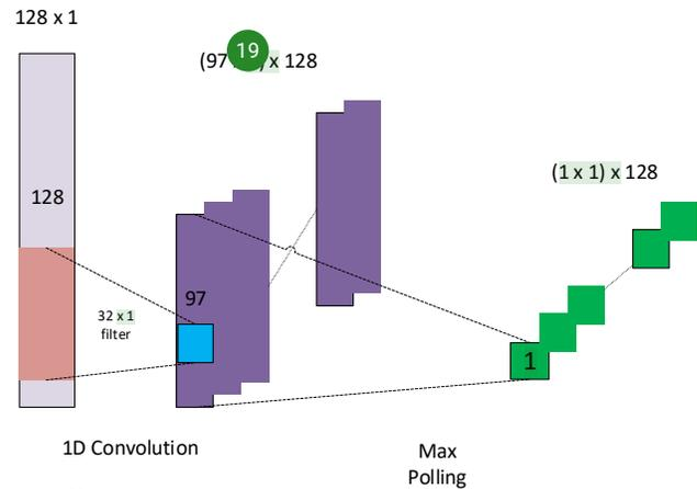
Fig. 2 1D-Convnet Structure for frame feature extraction [19]
