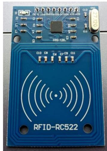
**Gambar 2.1. RFID MF RC522**
