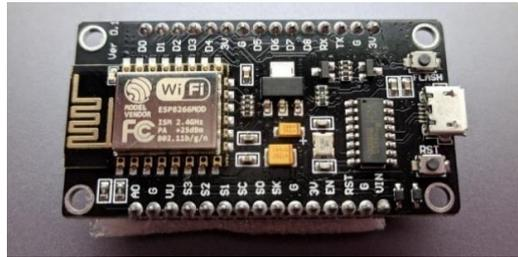
**Gambar 2.2. NodeMCU ESP8266 V3**
