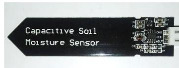
Gambar 2. 4 *Capacitive Soil Moisture Sensor* SEN0193
