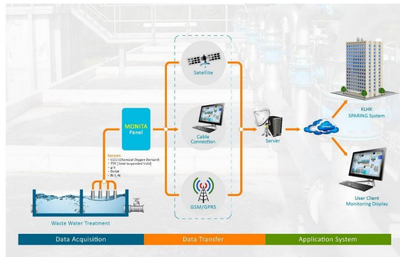
Gambar 5. Bagan Water Quality Monitoring System (Onlimo/SPARING)
