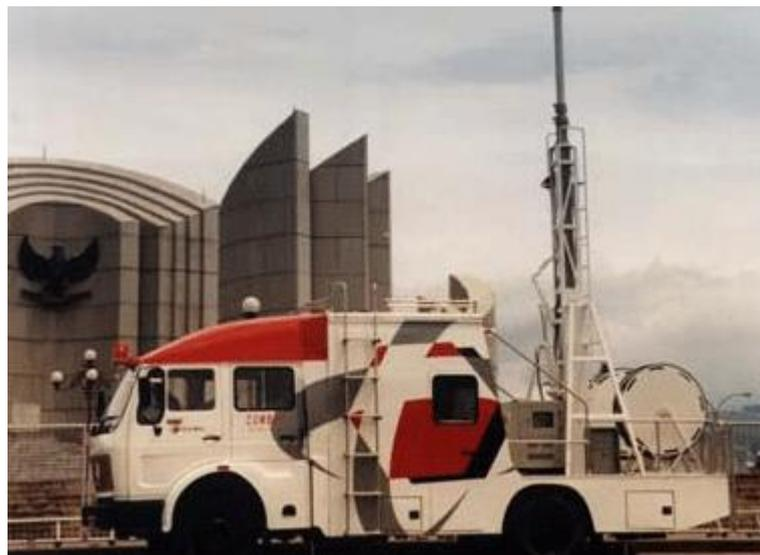
Gambar 2. 23 *Mobile Tower on Trailer*
