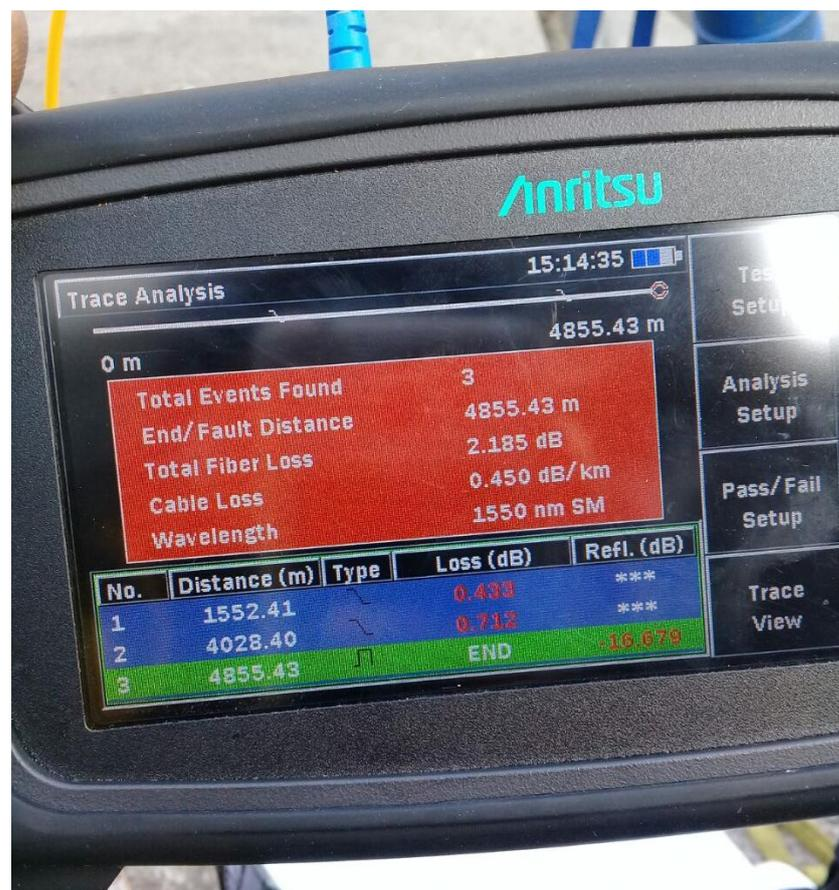
Gambar 2.2 *Optical Time Domain Reflection*
