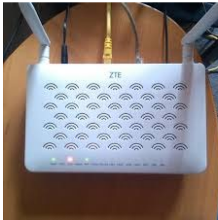
Gambar 2.10. Loss Signal Router
