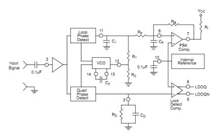
Figure 11. RFSK Demodulator circuit
