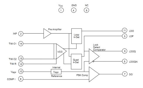
Figure 4. Block diagram for Demodulator XR2211
