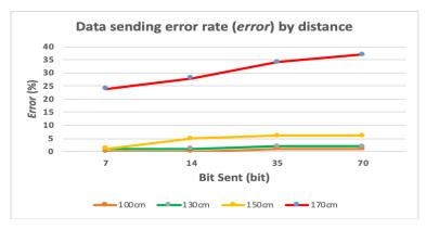
Figure 16. Graph of Dara sending error rate by distance
