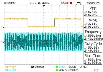
Figure 13. Modulator input and output measurement
