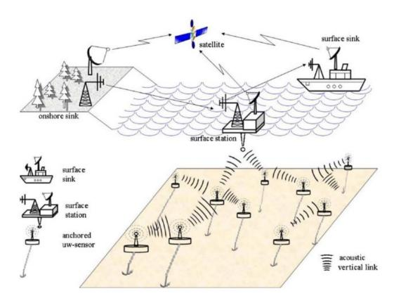
Figure 1. Underwater sensor network architecture (Akyildiz et al., 2005)
