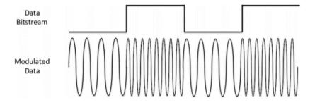
Figure 2. An FSK modulation
