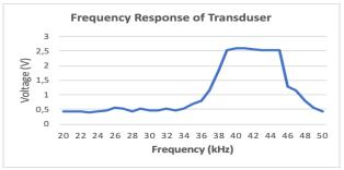
Figure 8. Transducer's Frequency Response graph
