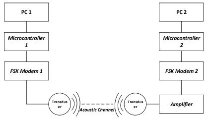
Figure 6. System Block Diagram
