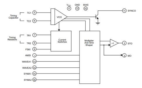
Figure 3. Block diagram of Modulator XR2206
