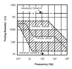
Figure 10. Resistor values proportional to oscillation frequency
