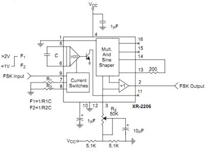
Figure 9. FSK Modulator circuit
