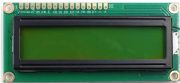
Gambar 2.8 Liquid Crystal Display 16x2[21].
