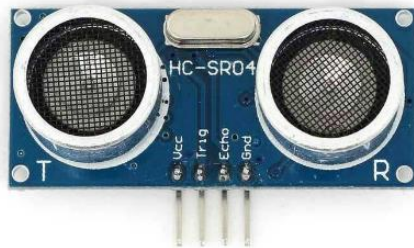
Gambar 2.6 Sensor Ultrasonik HC-SR04[19].
