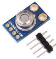
Gambar 2.5 Sensor Suhu MLX 90614 ( Infrared ) [18].
