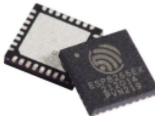
**Gambar 2.4 NodeMCU ESP8266 Chip**
