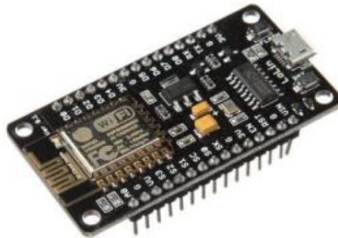
**Gambar 2.3 NodeMCU ESP8266**
