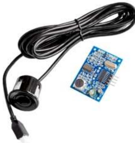
Gambar 2.2 Sensor Ultrasonik JSN-SR04T
