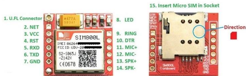
Gambar 2.8 SIM800L Pinout [15]
