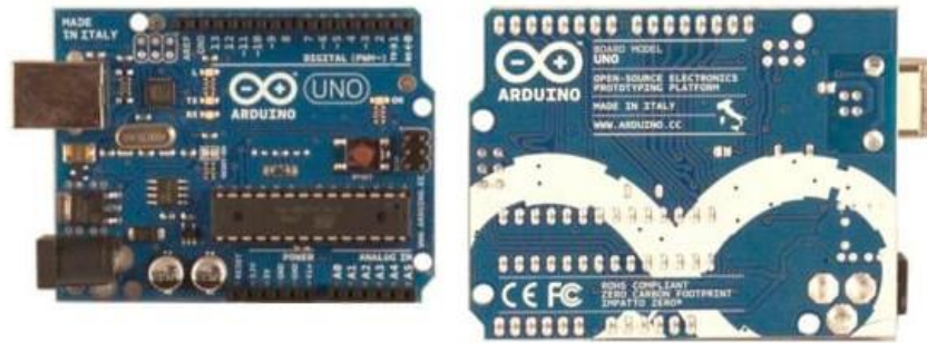
Gambar 2.5 Board Arduino Uno depan dan belakang [20]
