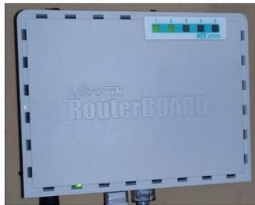
Gambar 2.20 *Mikrotik RB750Gr2*
