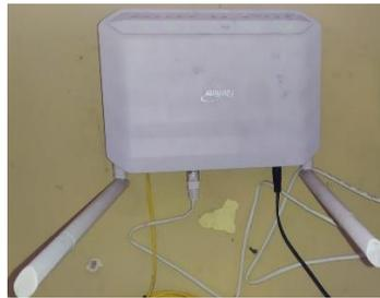
Gambar 2.18 Modem GPON HG6243C
