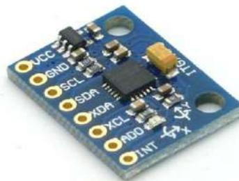
**Gambar 2.2** Sensor Akseleromer MPU6050[13].
