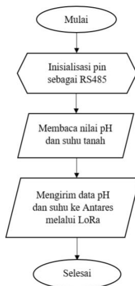
Gambar 3.5 Flowchart Perancangan Software
