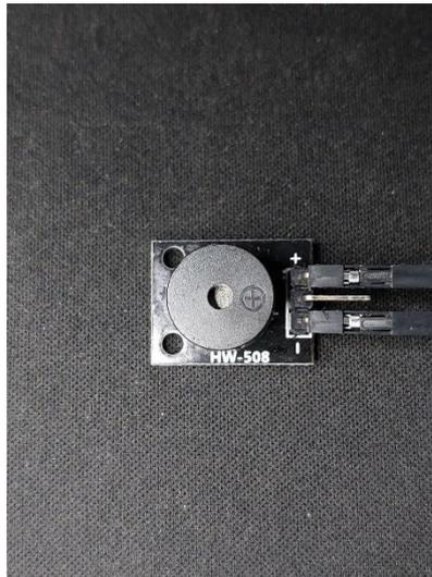
Gambar 2.5 Modul Buzzer KY-012
