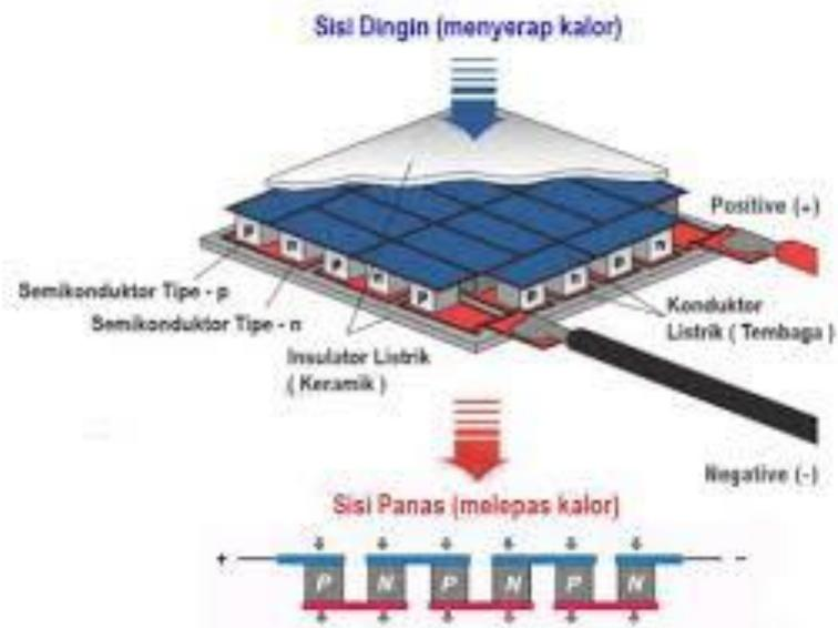
Gambar 2.1 Skema Aliran Peltier
