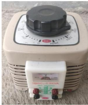
Gambar 2.9 Trafo Adjust Voltage
