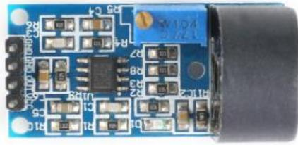
Gambar 2.6 Sensor Arus ZMCT103C[16]
