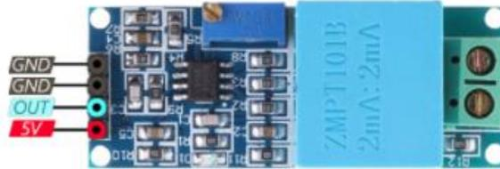
Gambar 2.5 Sensor Tegangan ZMPT101B[13]
