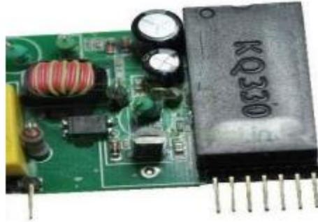
Gambar 2.2 Modul Power Line Communication KQ330
