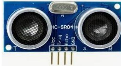
**Gambar 2.3 Sensor Ultrasonik (HC-SR04) [18]**
