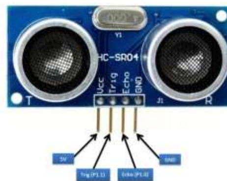
Gambar 2.3 Sensor Ultrasonik HC-SR04 [11]
