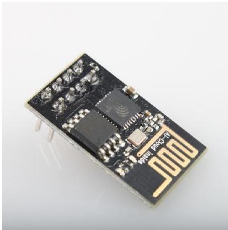
Figure 3 [Module Pin Counts, 8 pin, 14.3 mm *24.8 mm *3.0 mm]
