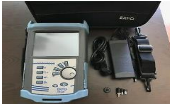
Gambar 3.1 Optical time Domain Reflectometer EXFO FTB-200
