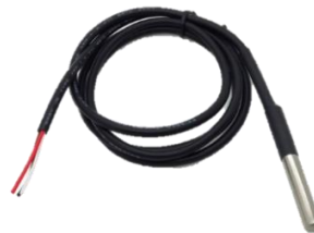
Gambar 3.12 Sensor Suhu Air ( DS18B20 )
