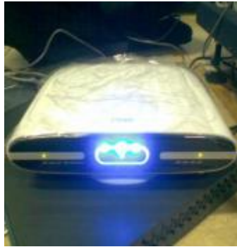
Gambar 2.20 Optical Network Termination/Unit (ONT/ONU) [13]
