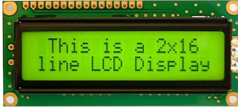
Gambar 2.11. tampilan LCD 2x16 [7] .
