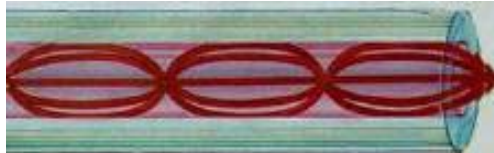
Gambar 1.3 Perambatan Gelombang Multi Mode Fibers [2]
