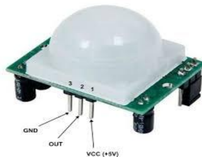
Gambar 2.9 Pin Sensor PIR
