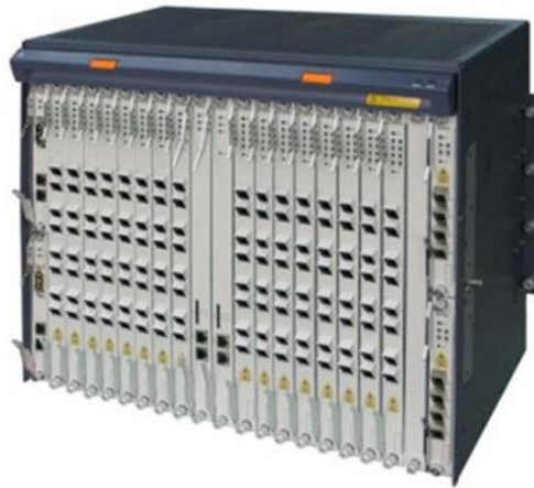
Gambar 2.12 Optical Line Terminal (OLT) [12]
