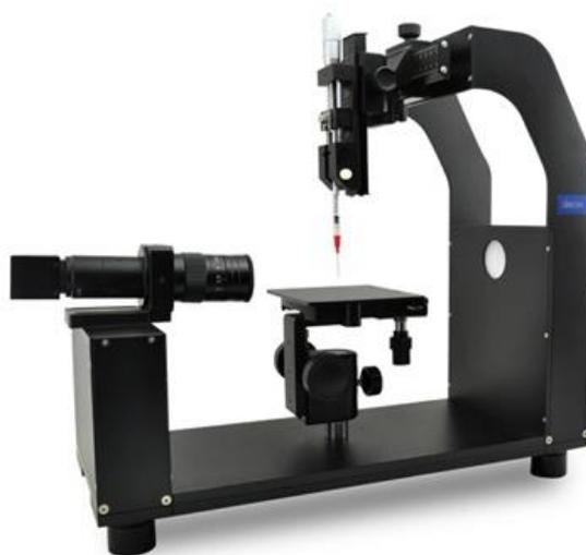
**Gambar 2. 7 Alat Uji Contact angle**
