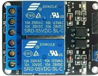
Gambar 9. Relay 2 Channel
