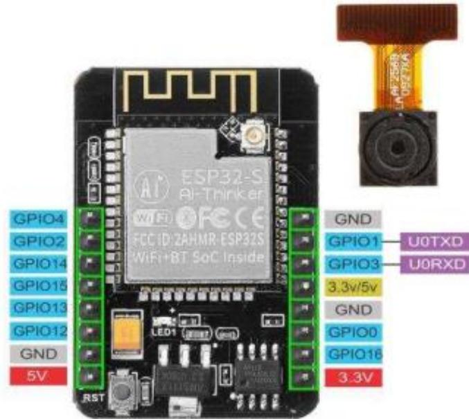
Gambar 2. 2 ESP32-CAM [31]
