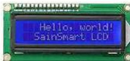
**Gambar 2.11** *LCD crystal 16 x 2* [31]
