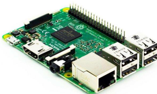
Gambar 2.23 Board Raspberry Pi [34]
