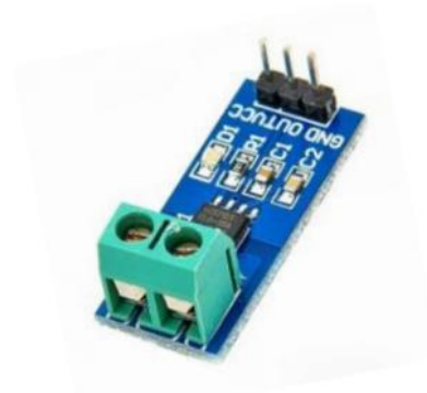
Gambar 2. 3 Sensor arus ACS712 [21].
