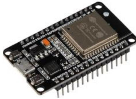
**Gambar 2.3 NodeMCU ESP32**
