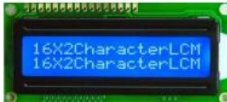
**Gambar 2.7 LCD 16x2**
