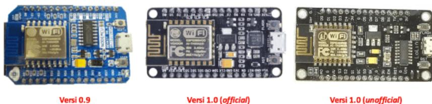
Gambar 2. 3 NodeMCU ESP8266 [22]
