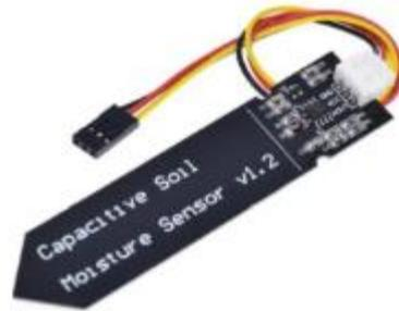
**Gambar 2. 4 Sensor Soil moisture v1.2 [24]**
