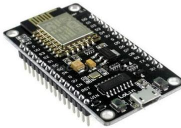
**Gambar 3.7 NodeMCU ESP8266**
