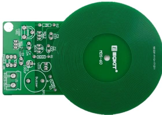
**Gambar 2.3 Sensor *Kit Diy Metal Detector* [15]**
