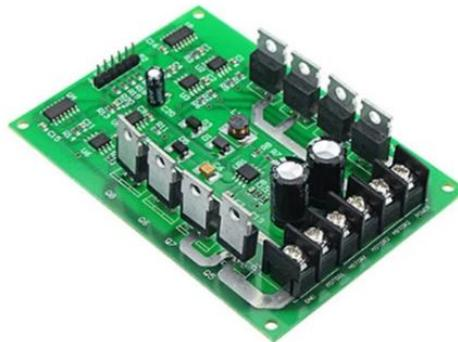
**Gambar 3.6 *Module H-bridge MOSFET IRF3205***
