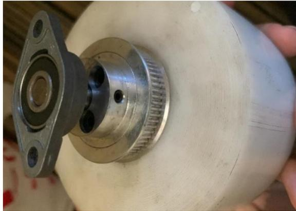
**Gambar 3.7** Roda berbahan *Polytetrafluoroethylene (PTFE)*
