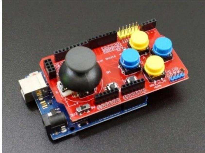
**Gambar 3.5 Joystick Shield v1.a Funduino**
